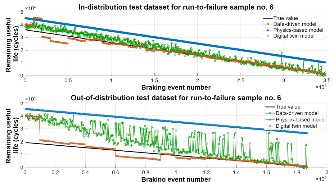
Figure 12. Remaining useful life estimates for the data-driven, physics-based, and digital-twin models. The top plot shows an in-distribution test sample with typical degradation behaviour, while the bottom plot shows an out-of-distribution sample with accelerated wear.
