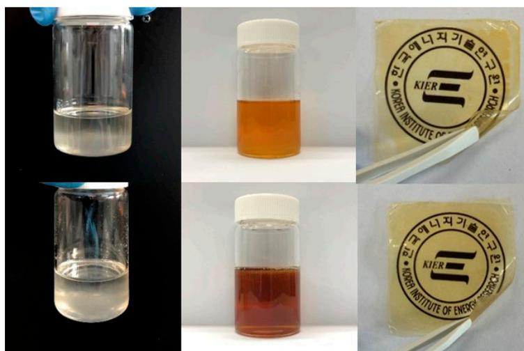
**Figure 2.** Photographic images of the Nafion-TMA (trimethyl amine, upper) and Aquivion-TMA (lower)-based dispersions in *N,N*-dimethylformamide (DMF, left) and *N*-methyl-2-pyrrolidone (NMP, middle), and the resulting membranes (right).
