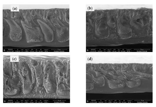
**Figure 4.** Cross-sectional membrane sheets observed by SEM (2000 × magnification): (a) Pristine CA membrane (DMAc); (b) 1.0 wt% CPHE/CA composite membrane (DMAc); (c) Pristine CA membrane (DMF); and (d) 1.0 wt% CPHE/CA composite membrane (DMF).
