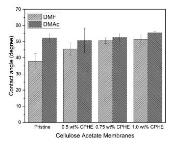
Figure 5. Hydrophilicity of the cellulose acetate membrane sheets.
