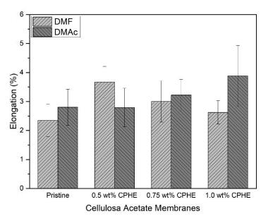
Figure 7. Elongation of the membrane sheets.
