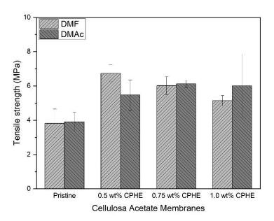
Figure 6. Tensile strength of the cellulose acetate membrane sheets.
