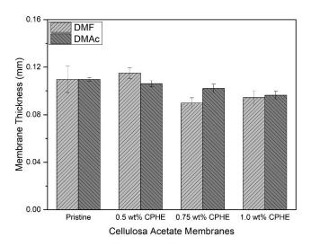
**Figure 3.** Average membrane thickness with different membrane variations.
