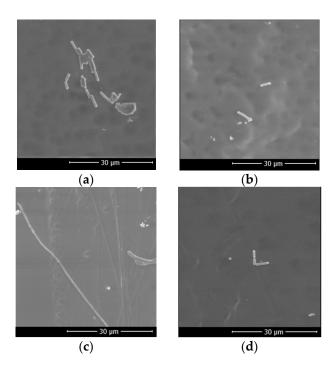
**Figure 9.** *Escherichia coli* attachment to the membrane surface: (a) Pristine CA membrane (DMAc); (b) 1.0 wt% CPHE/CA composite membrane (DMAc), (c) Pristine CA membrane (DMF) (d) 1.0 wt% CPHE/CA composite membrane (DMF).
