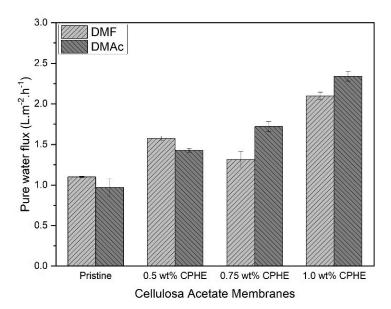
Figure 8. Pure water flux measured on each membrane.
