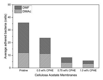
**Figure 10.** Number of bacteria attached to the membrane.
