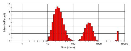
Figure 2. Particle size and distribution of the CPHE phenolic nanopowder.
