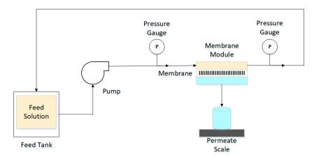
Figure 1. Crossflow membrane filtration system.
