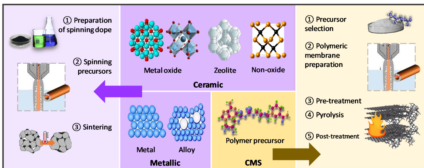
Figure 7. The categorization and preparation routes of inorganic hollow fiber membranes.
