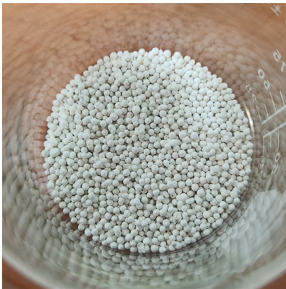
Scheme 1. PES microspheres mounted with \text{TiO}_2 photocatalyst.
