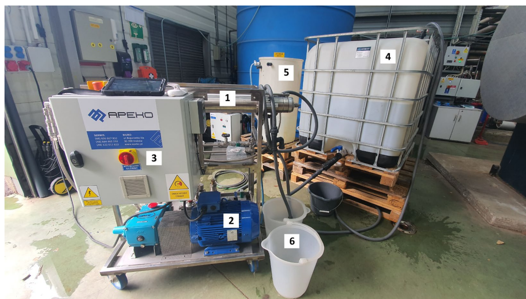
Figure 1. View of the APEKO UF-1 pilot-scale installation. 1—Cylindrical PCI B1 module equipped with 18 membrane elements; 2—CAT high-pressure recirculation pump; 3—Electrical control box with operating panel; 4—1000 L IBC tank containing wastewater feed for ultrafiltration; 5—Cleaning chemical tank; 6—Reference permeate container.
