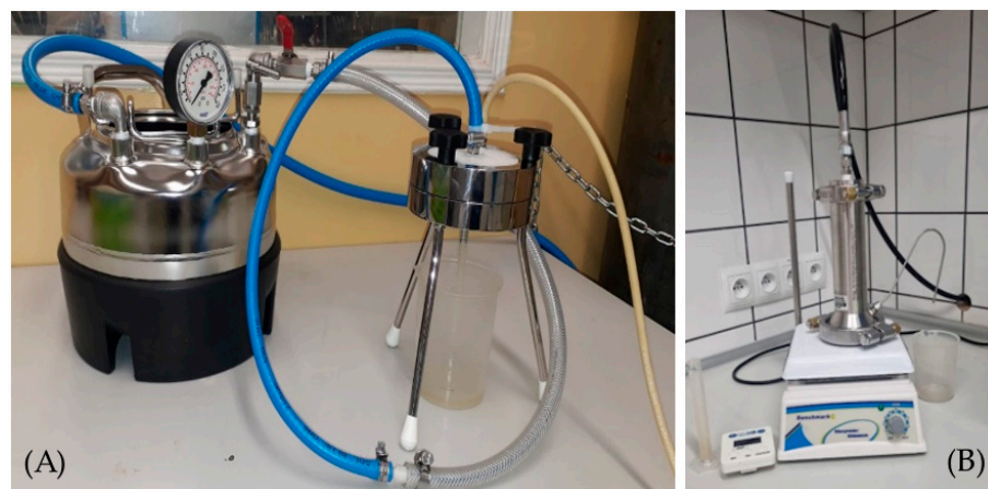
Figure 1. Filtration systems: (A) Sterlitech laboratory system with ceramic membranes; (B) Sterlitech high-pressure cell.
