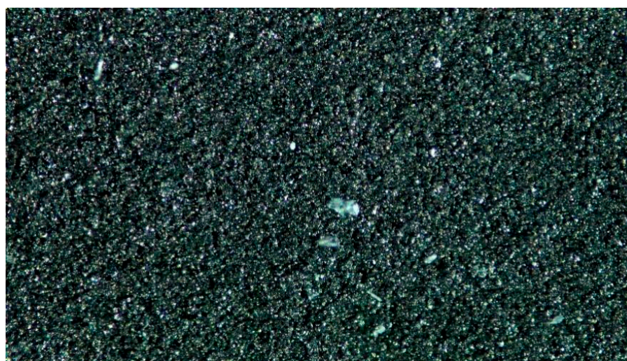
Figure 2. SEM image of the cathode activated carbon electrode surface.
