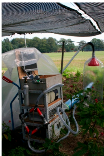
Figure 12. Transportable facility to label plants in the field with ^{13}\text{CO}_2 . The specific example shows an experiment with Panax ginseng plants aimed to elucidate the biosynthesis of ginsenosides.
