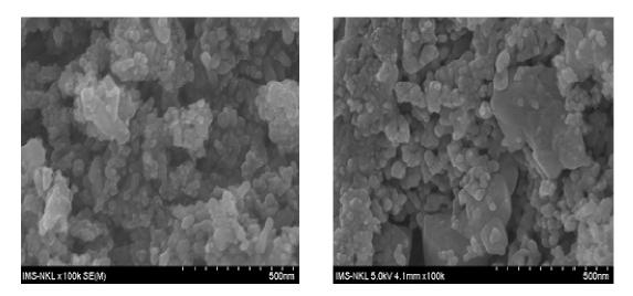
Figure 6. SEM images of ZrO<sub>2</sub> product after SE by PC88A/toluene.
