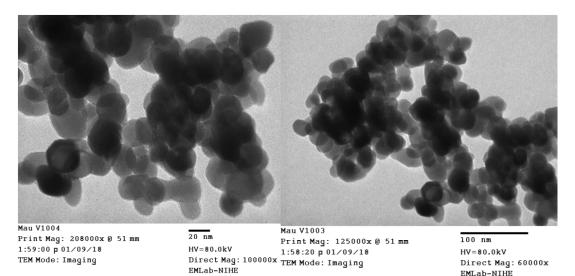
Figure 7. TEM images of ZrO<sub>2</sub> product after SE by PC88A/toluene.
