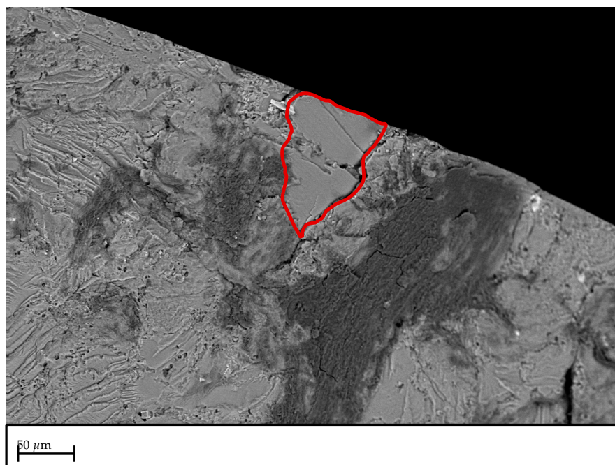
Figure 11. Representative fracture-initiating slipplane at Pos#1.
