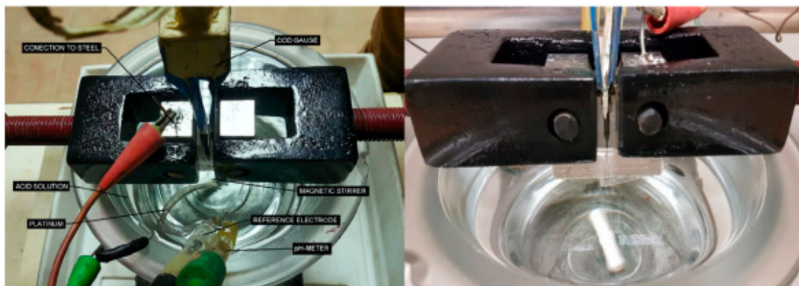
Figure 12. Set-up of the slow rate tests in environment using C(T) specimens.
