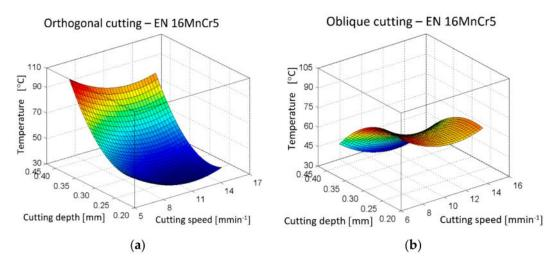
**Figure 8.** The dependence of temperature T on cutting speed  $v_c$  and cutting depth  $a_p$ , (a) Orthogonal cutting; (b) oblique cutting.
