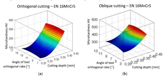
**Figure 15.** Dependency of microhardness HV on the cutting depth  $a_p$  and on the orthogonal rake angle  $\gamma_0$ . (a) Orthogonal cutting; (b) oblique cutting.
