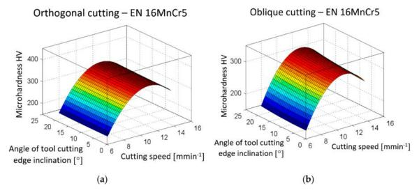
**Figure 14.** Dependency of microhardness HV on the cutting speed  $v_c$  and on the angle of tool cutting edge inclination  $\lambda_s$ . (a) Orthogonal cutting; (b) oblique cutting.
