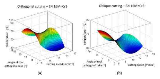
**Figure 9.** The dependence of temperature T on cutting speed  $v_c$  and angle of tool orthogonal rake  $\gamma_o$ . (a) Orthogonal cutting; (b) oblique cutting.
