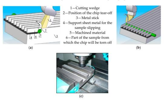
**Figure 5.** The principle of the designed method for instantaneous contact interruption between a tool and workpiece showing (a) orthogonal cutting, (b) oblique cutting, (c) real workpiece.
