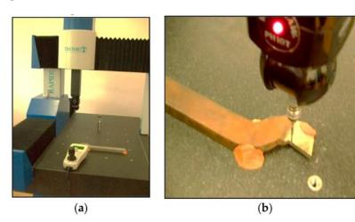
**Figure 3.** Preliminary tests of input angles of tool orthogonal rake  $\gamma_0$ , (a) Overall view on the testing equipment RAPID CNC THOME, (b) Detail view on the measuring of a tool orthogonal rage angle.
