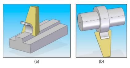
Figure 1. The principle of orthogonal cutting in (a) planing and (b) turning.
