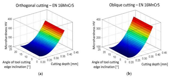
**Figure 16.** Dependency of microhardness HV on the cutting depth  $a_p$  and on the angle of tool cutting edge inclination  $\lambda_{s.}$  (**a**) Orthogonal cutting; (**b**) oblique cutting.
