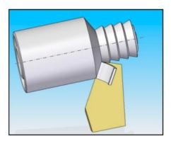
Figure 2. The principle of oblique cutting.
