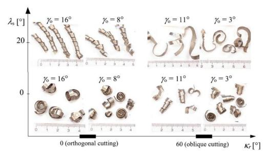
**Figure 7.** The shapes of chips of EN 16MnCr5 steel and their dependence on tool cutting edge angle  $\kappa_r$ , angle of tool cutting edge inclination  $\lambda_s$ , and angle of tool orthogonal rake  $\gamma_0$  at  $a_v = 0.2$  mm,  $v_c = 15$  mmin<sup>-1</sup>.
