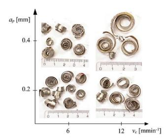
**Figure 6.** The shapes of chips and their dependence on cutting speed  $v_c$  and cutting depth  $a_p$  at tool angles for  $\gamma_0 = 16^\circ$ ,  $\lambda_s = 0^\circ$ ,  $\kappa_r = 0^\circ$ .
