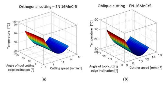
**Figure 10.** The dependence of temperature T on cutting speed  $v_c$  and angle of tool cutting edge inclination  $\lambda_s$ . (a) Orthogonal cutting; (b) oblique cutting.
