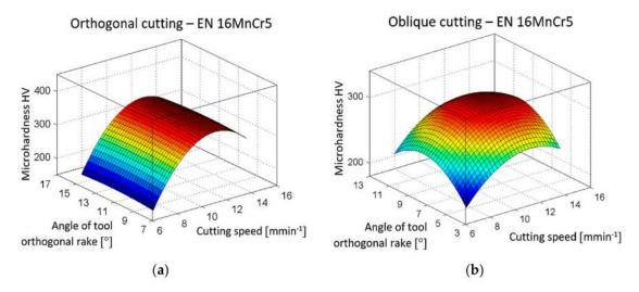
**Figure 13.** Dependency of microhardness HV on the cutting speed  $v_c$  and on the orthogonal rake angle  $\gamma_0$ . (a) Orthogonal cutting; (b) oblique cutting.
