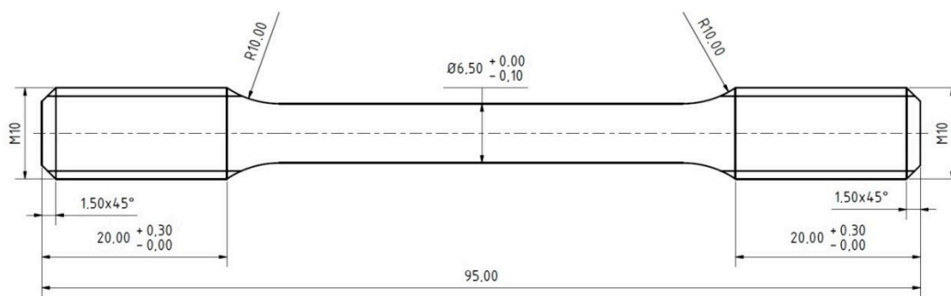
Figure 8. Samples used to measure mechanical properties as exposed in a vacuum furnace (unit: mm).
