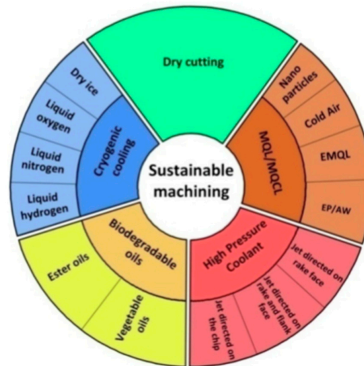
Figure 7. Wheel of sustainable machining. Reproduced from [53], with permission from Elsevier, 2019.
