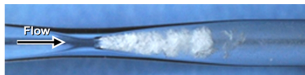
Figure 2. Aspect of cavitation through Venturi tube [47].
