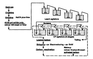
**Figure 1.** Diagram of gold cyanide leaching using activated carbon recovery. Reproduced and adapted from [9], with permission from PERGAMON, 1987.
