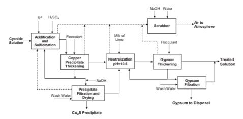
**Figure 6.** SART process flowsheet. Reproduced and adapted from [16], with permission from PERGAMON, 2020.
