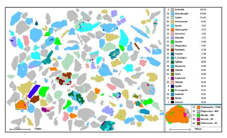
**Figure 4.** Image containing copper sulfide minerals. Reproduced and adapted from [13], with permission from the authors, 2020.
