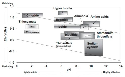
**Figure 5.** Diagram showing the typical range of operation of lixiviants. Reproduced and adapted from [22], with the permission from Elsevier B.V., 2016.
