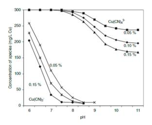
**Figure 2.** Comparison of cyanide species vs. pH. Reproduced and adapted from [8], with permission from Elservier B.V., 2005.
