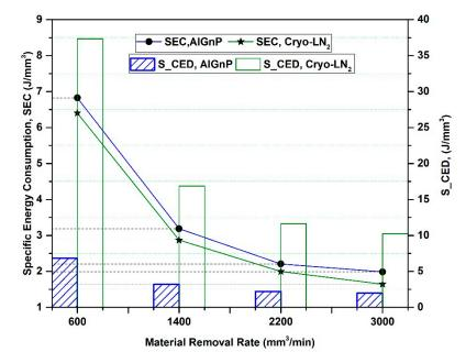
**Figure 11.** Influence of *MRR* on specific energy consumption (SEC) and specific cumulative energy demand (S\_CED) under both environments ( $a_p = 0.8 \text{ mm}$ ; f = 0.1 mm/rev; P = 0.5 MPa;  $n_p = 1.2$ ).
