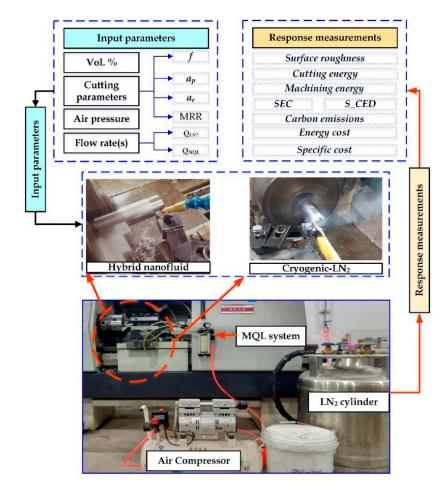
Figure 3. Experimental setup for hybrid nanofluid and cryogenic LN<sub>2</sub> approaches.
