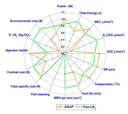
**Figure 15.** Radar graph to evaluate overall process performance ( $a_p = 0.8 \text{ mm}$ ; f = 0.1 mm/rev; P = 0.5 MPa;  $v_c = 150 \text{ m/min}$ ).
