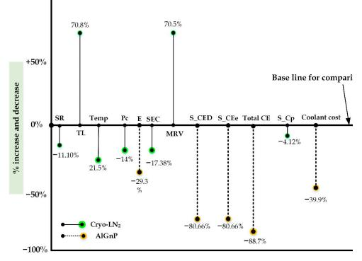
**Figure 14.** A holistic comparison between hybrid Al-GnP and cryogenic LN<sub>2</sub> at higher cutting conditions  $(a_p = 0.8 \text{ mm}; f = 0.1 \text{ mm/rev}; P = 0.5 \text{ MPa}; v_c = 150 \text{ m/min}).$
