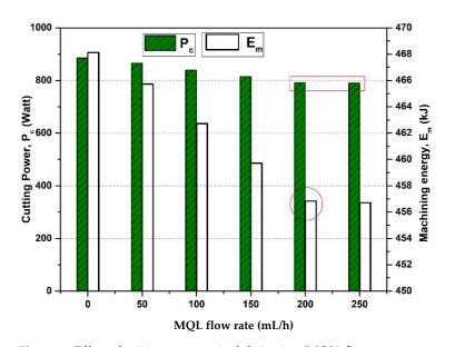
**Figure 5.** Effect of minimum quantity lubrication (MQL) flow rate on power and energy consumption ( $v_c = 70 \text{ m/min}$ ,  $a_p = 0.8 \text{ mm}$ ; f = 0.1 mm/rev; Pp = 0.5 MPa).
