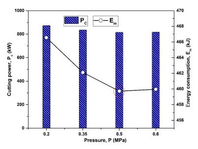
**Figure 6.** Effect of mist pressure on energy and power consumption ( $v_c = 70 \text{ m/min}$ ,  $a_p = 0.8 \text{ mm}$ ; f = 0.1 mm/rev;  $n_p = 1.2$ ).
