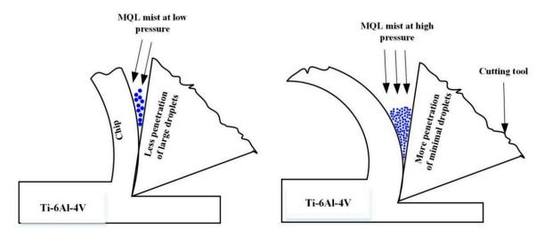
Figure 7. Effect of air pressure on airdrops at the machining zone.
