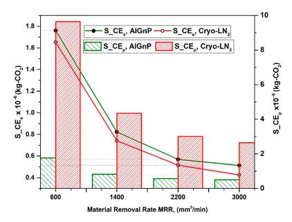
**Figure 12.** Influence of *MRR* on carbon footprint of electrical energy consumption and CO<sub>2</sub> emissions per part ( $a_p = 0.8 \text{ mm}$ ; f = 0.1 mm/rev; p = 0.5 MPa;  $n_p = 1.2$ ).
