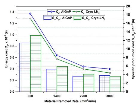
**Figure 13.** Comparison of energy cost and specific production cost under two various cooling/lubrication approaches ( $a_p = 0.2 \text{ mm}$ ; f = 0.1 mm/rev; p = 0.5 MPa;  $n_p = 1.2$ ).
