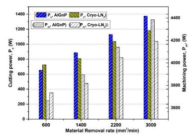
**Figure 10.** Effect of increasing material removal rate (*MRR*) on cutting power and machining energy in Al-GnP-assisted machining and cryogenic LN<sub>2</sub>-assisted machining  $(a_p = 0.8 \text{ mm}; f = 0.1 \text{ mm/rev}; P = 0.5 \text{ MPa}; n_p = 1.2).$
