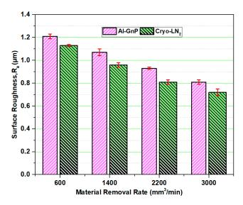
**Figure 9.** Comparison of the surface quality of workpieces under hybrid nanofluid- and cryogenic LN<sub>2</sub>-assisted machining processes ( $a_p = 0.8 \text{ mm}$ ; f = 0.1 mm/rev; P = 0.5 MPa;  $n_p = 1.2$ ).
