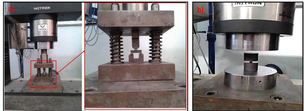
**Figure 4.** (a) The three-point bending setup, with an enlarged image of the measurement of the Transverse rupture strength (TRS) of the cemented carbide materials. (b) The compression-test system.
