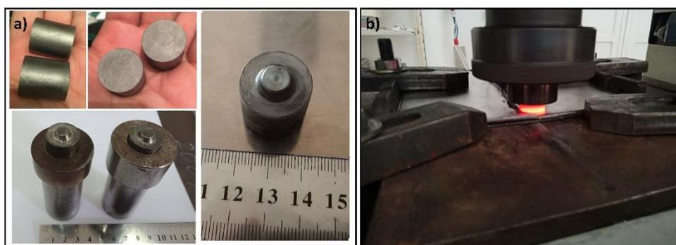
**Figure 16.** The manufactured cylindrical parts from the WC-based composites with 5 wt% Ni and 2.5 wt%  $Y_2O_3$  for the FSW tool applications. (a) Images of the parts after consolidation, grinding for the required geometries and insertion in the tool steel holder. (b) The FSW tool during the welding of the Ni base alloy.
