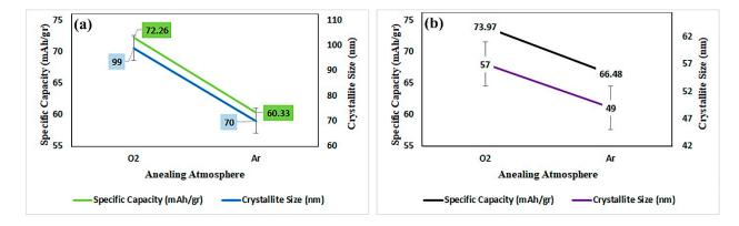
**Figure 3.** Comparison of the effect of annealing atmosphere on the crystal grain sizes and the specific capacity obtained X-ray diffraction data using the Williamson–Hall equation (**a**) TiNb<sub>2</sub>O<sub>7</sub>, (**b**) Ti<sub>2</sub>Nb<sub>10</sub>O<sub>29</sub>.
