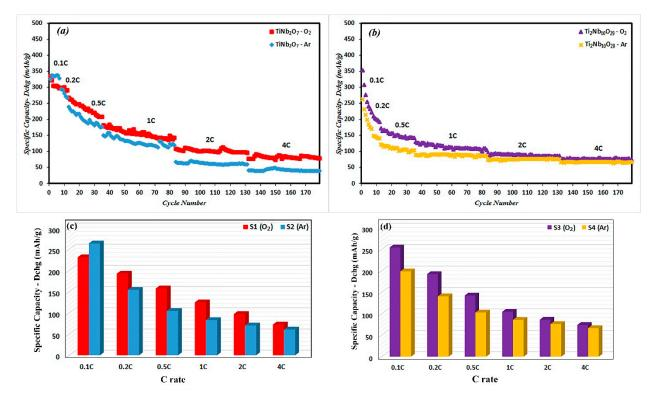
**Figure 5.** Cycling performance of the Electrodes synthesized in different atmospheres at various charge/discharge rates as indicated (**a**) TiNb<sub>2</sub>O<sub>7</sub>, (**b**) Ti<sub>2</sub>Nb<sub>10</sub>O<sub>29</sub>, (**c**,**d**) bar charts for comparing the discharge capacities at different C rates.
