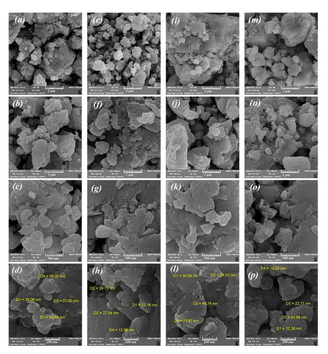
**Figure 1.** Images of FESEM microscope from the samples: (**a**–**d**) S1, (**e**–**h**) S2, (**i**–**l**) S3, and (**m**–**p**) S4 synthesized by ball milling under annealing treatment.
