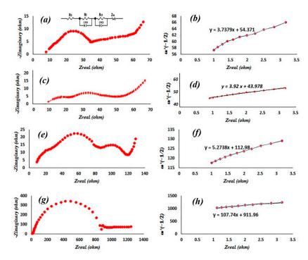
**Figure 6.** EIS spectra of TiNb<sub>2</sub>O<sub>7</sub> and Ti<sub>2</sub>Nb<sub>10</sub>O<sub>29</sub> annealed under different atmospheres (**a**,**e**) oxygen atmosphere, (**c**,**g**) argon atmosphere, and equivalent circuit for fitting experimental data, (**b**,**d**,**f**,**h**) the relationship between Z' and the square root of frequency ( $\omega$ -1/2) in the low-frequency region for TiNb<sub>2</sub>O<sub>7</sub> and Ti<sub>2</sub>Nb<sub>10</sub>O<sub>29</sub>.
