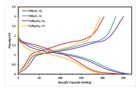
**Figure 4.** Charge/discharge curves of two synthesized samples in different atmospheres at 0.1 C cycled between 0 and 3 V.
