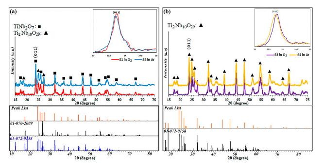
**Figure 2.** Diffracted X-ray patterns of the  $TiNb_2O_7$  and  $Ti_2Nb_{10}O_{29}$  compounds, annealed under different atmospheres (**a**) Peak shift of the (011) plane composition  $TiNb_2O_7$  and (**b**) Peak shift of the (011) plane composition  $Ti_2Nb_{10}O_{29}$ .
