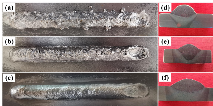
Figure 2. Bead-on-plate welds appearance and cross section of different welding. (a,d) UWW; (b,e) WG-USAW; (c,f) EP-USAW.
