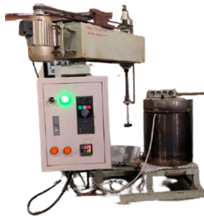
Figure 5. Stir casting setup.
