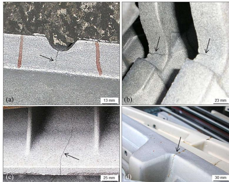
**Figure 63.** Different locations of hot tears found in some large extended grey iron castings (a–d).
