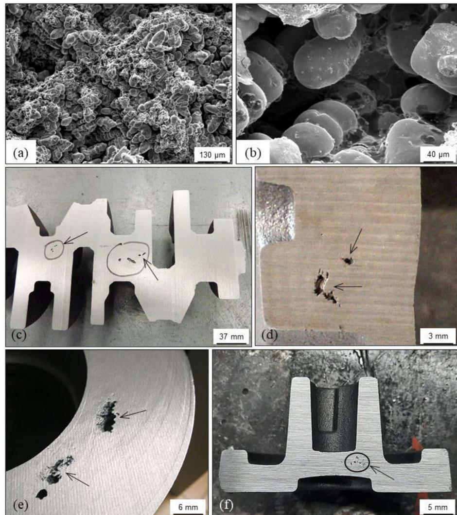
**Figure 72.** (a,b) SEM images of internal surfaces in a secondary shrinkage defect found in a ductile iron casting; (c–f) defects located in last solidification areas.
