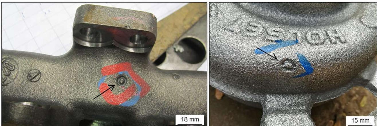
**Figure 53.** Areas of castings showing fish-eye defects.
