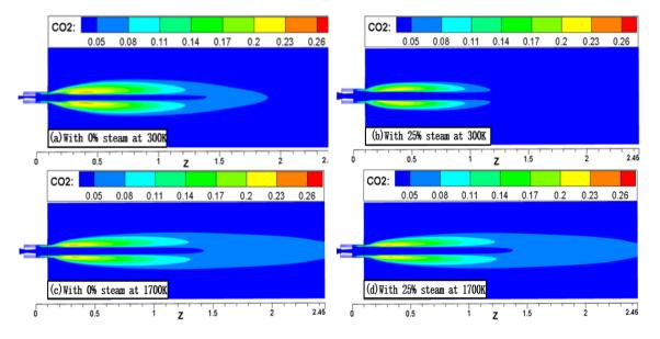
**Figure 18.** Longitudinal cross-sectional distributions of CO<sub>2</sub> in the coherent supersonic jets under different conditions: (**a**) 0% steam and 100% oxygen at 300 K; (**b**) 25% steam and 75% oxygen at 300 K; (**c**) 0% steam and 100% oxygen at 1700 K; and (**d**) 25% steam and 75% oxygen at 1700 K.
