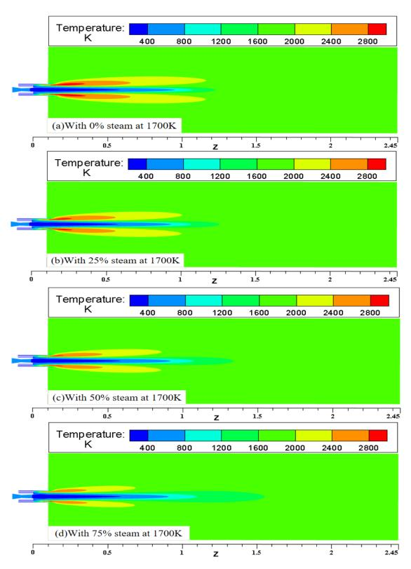
**Figure 11.** Total temperature distributions of the  $H_2O$  and  $O_2$  mixed jets in the longitudinal section at an ambient temperature of 1700 K under various conditions: (**a**) 0% steam and 100% oxygen; (**b**) 25% steam and 75% oxygen; (**c**) 50% steam and 50% oxygen; and (**d**) 75% steam and 25% oxygen.
