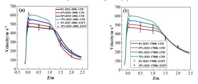
**Figure 5.** The axial velocity distribution on the centerline of coherent supersonic jet. (**a**) The velocity measured by numerical simulations and experimentally at 300 K. (**b**) The velocity value measured by numerical simulations and experimentally at 1700 K.
