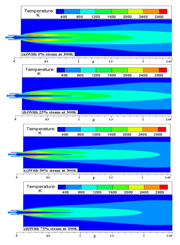
**Figure 10.** Total temperature distributions of the  $H_2O$  and  $O_2$  mixed jets in the longitudinal section at an ambient temperature of 300 K under various conditions: (a) 0% steam and 100% oxygen; (b) 25% steam and 75% oxygen; (c) 50% steam and 50% oxygen; and (d) 75% steam and 25% oxygen.
