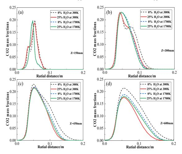
**Figure 17.** Radial distribution of the CO<sub>2</sub> mass fraction at different positions from the spray gun outlet at 300 and 1700 K: (**a**) Z = 150 mm, (**b**) Z = 300 mm, (**c**) Z = 150 mm, and (**d**) Z = 600 mm.
