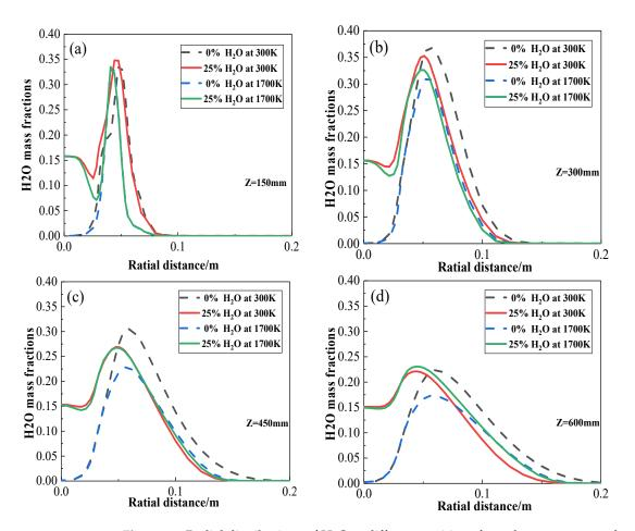
**Figure 15.** Radial distributions of  $H_2O$  at different positions from the spray gun outlet at 300 and 1700 K: (a) Z = 150 mm, (b) Z = 300 mm, (c) Z = 150 mm, and (d) Z = 600 mm.
