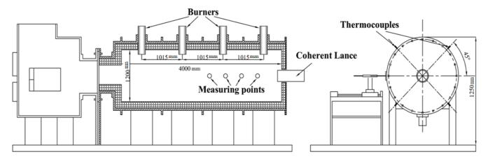
Figure 2. Schematic diagram of the combustion furnace.
