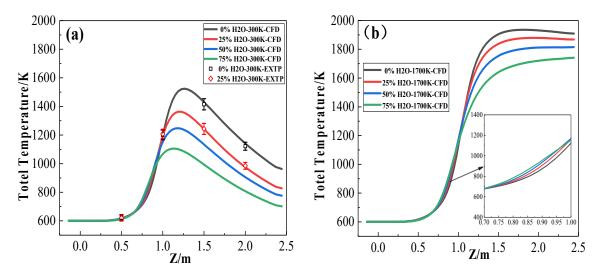
**Figure 9.** The total temperature distribution of the  $H_2O$  and  $O_2$  mixed injection jet along the axis. (a) The temperature distribution of the mixed injection jet with different components at an ambient temperature of 300 K. (b) The temperature distribution of the mixed injection jet with different components at an ambient temperature of 1700 K.
