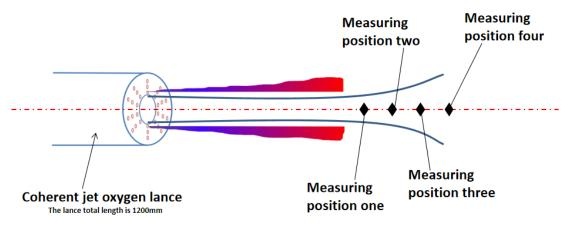
**Figure 1.** Schematic diagram of the coherent supersonic jet and the experimental measurement principle.
