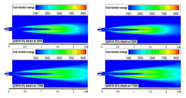
**Figure 13.** Axial cross-sectional distributions of the turbulent flow energy of the coherent supersonic jet at different temperatures and different water contents: (**a**) 0% steam and 100% oxygen at 300 K; (**b**) 25% steam and 75% oxygen at 300 K; (**c**) 0% steam and 100% oxygen at 1700 K; and (**d**) 25% steam and 75% oxygen at 1700 K.
