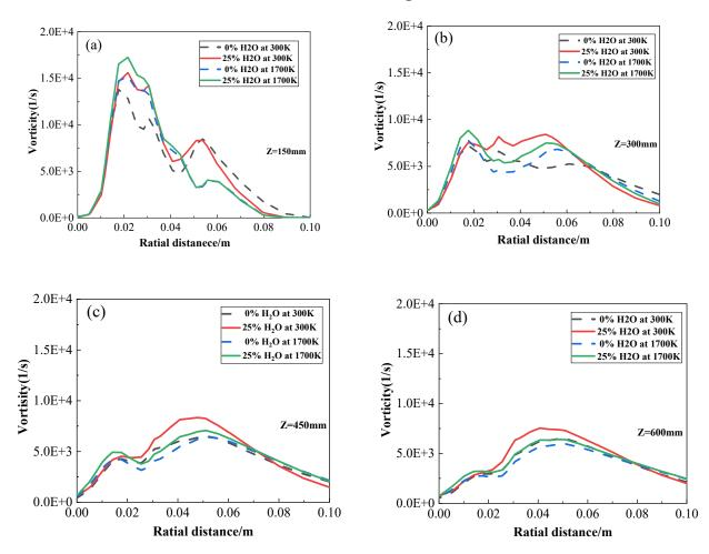
**Figure 12.** Radial distribution of the jet vorticity at different positions from the jet outlet under ambient temperatures of 300 and 1700 K: (**a**) Z = 150 mm, (**b**) Z = 300 mm, (**c**) Z = 150 mm, and (**d**) Z = 600 mm.
