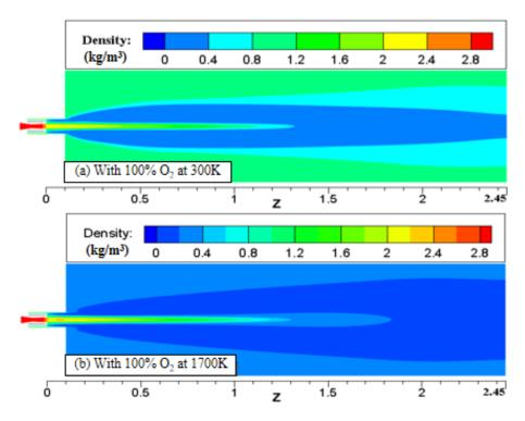
**Figure 8.** Density distribution of the full oxygen coherent supersonic jet at 300 and 1700 K. (**a**) The density distribution of the mixed injection jet at an ambient temperature of 300 K. (**b**) The density distribution of the mixed injection jet at an ambient temperature of 1700 K.
