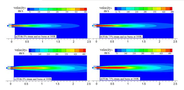
Figure 6. Axial velocity nephogram on the centerline of a coherent supersonic jet.
