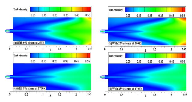
**Figure 14.** Axial cross-sectional distribution of the turbulent viscosity of the coherent supersonic jet at different temperatures and different water contents: (**a**) 0% steam and 100% oxygen at 300 K; (**b**) 25% steam and 75% oxygen at 300 K; (**c**) 0% steam and 100% oxygen at 1700 K; and (**d**) 25% steam and 75% oxygen at 1700 K.
