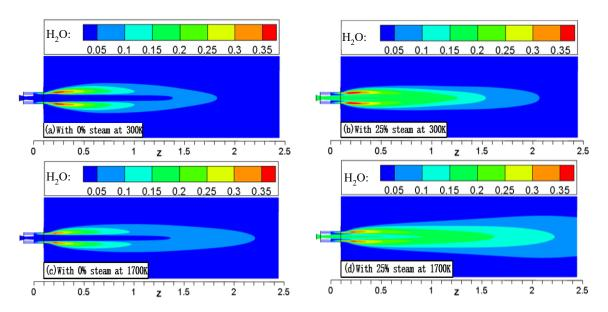
**Figure 16.** Longitudinal cross-sectional distributions of  $H_2O$  in the coherent supersonic jets under different conditions: (**a**) 0% steam and 100% oxygen at 300 K; (**b**) 25% steam and 75% oxygen at 300 K; (**c**) 0% steam and 100% oxygen at 1700 K; and (**d**) 25% steam and 75% oxygen at 1700 K.
