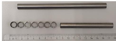
**Figure 2.** Cladding tube before hydrogenation (top) and after sectioning in 5 mm rings prior to desorption (bottom).
