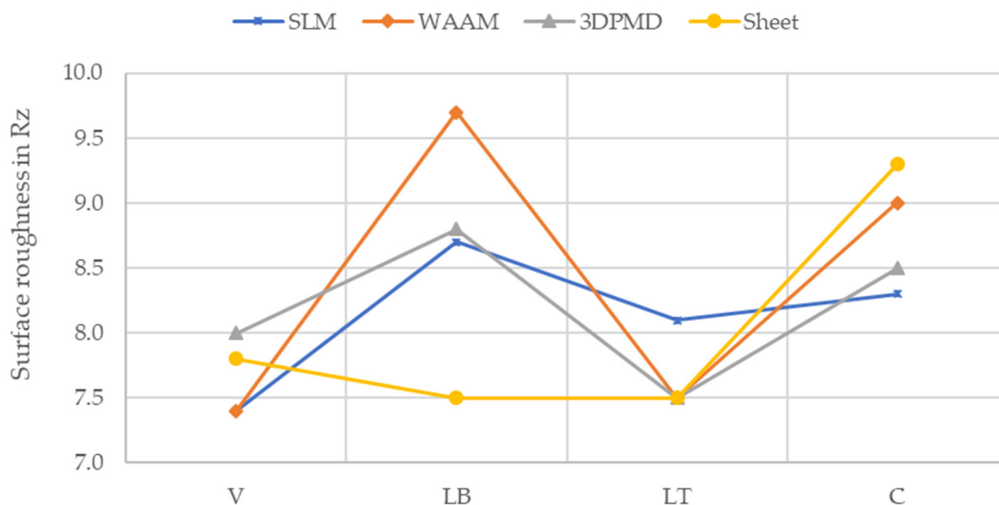
Figure 16. Rz values of the milled specimens by direction and AM process.
