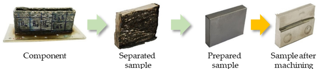
Figure 8. Sequence of sample preparation.
