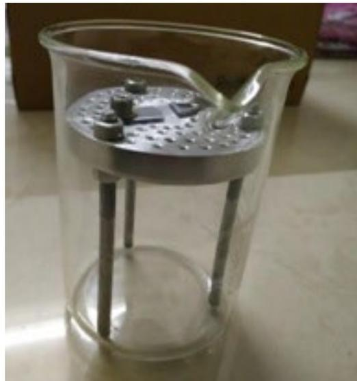
**Figure 1.** Liquid laser treatment experimental rig. Reprinted/adapted with permission from Ref. [42] 2021, Elsevier.
