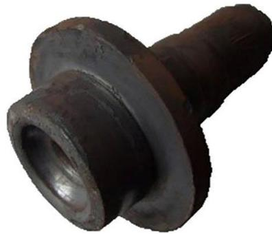
**Figure 22.** Results of hot extrusion experiment.
