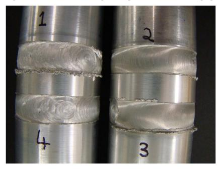
**Figure 15.** Visual inspection of the surfaces obtained from OFSW, reprinted with permission from [22], 2023, Elsevier.
