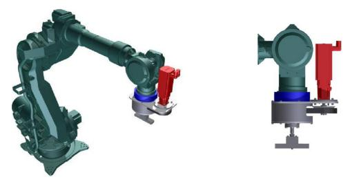
**Figure 10.** Articulated arm robot adapted for FSW, reprinted with permission from [54], 2023, Springer Nature.
