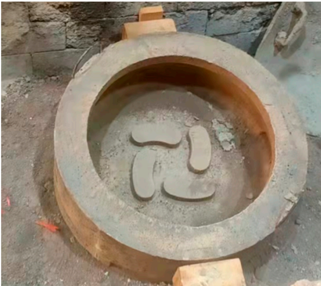
Figure 13. Turbulence inhibitor in the tundish after algorithm-assisted optimization.
