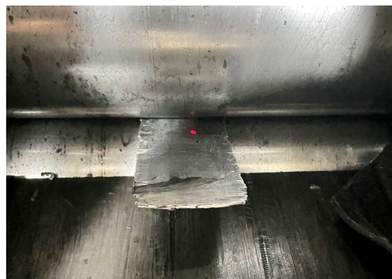
Figure 10. Aiming point of the pyrometer at the strip outlet section.
