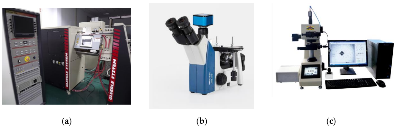
Figure 1. Experimental equipment and flow chart: (a) Gleeble-3500 thermal simulation testing machine; (b) IE500M metallographic microscope; (c) 430SVA Vickers hardness tester.
