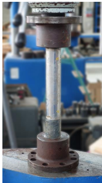
Figure 4. Flanges press-fitting of multi-track laser-hardened axle model.
