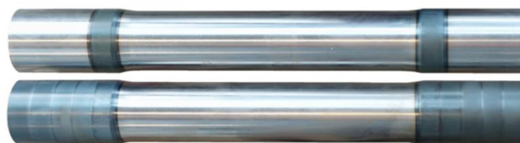
Figure 2. Axle models with single-track (up) and multi-track (down) laser hardening.
