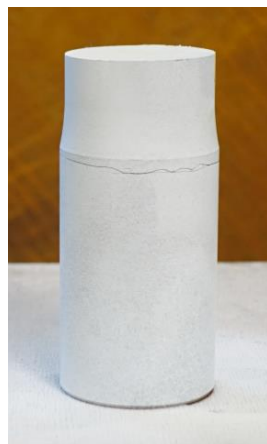
Figure 10. Representative axle seat after failure.
