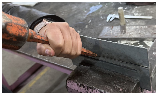
Figure 2. Chisel test performed in the lap joints.
