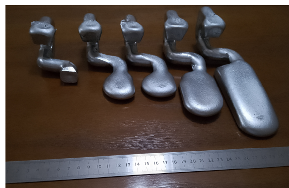
Figure 5. Runner and samples of rheocast A356 from left to right at 615 °C, 630 °C, 630 °C and 690 °C, respectively, made using horizontal SCP.
