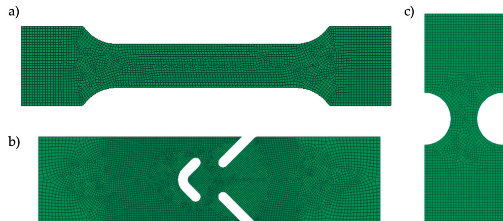
Figure 4. Image of the sample meshing of each sample. (a) Conventional tensile sample, (b) shear sample, (c) notched sample.
