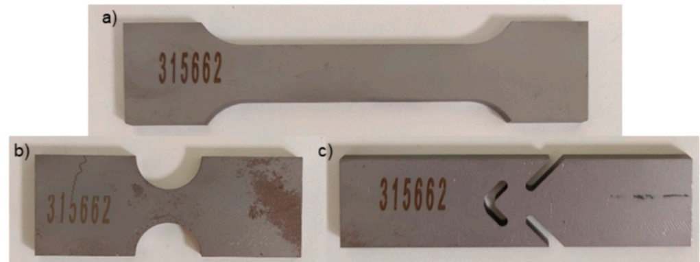
Figure 2. Image of the samples that were employed in the tensile tests. (a) Conventional tensile test, (b) notched sample, (c) shear sample.
