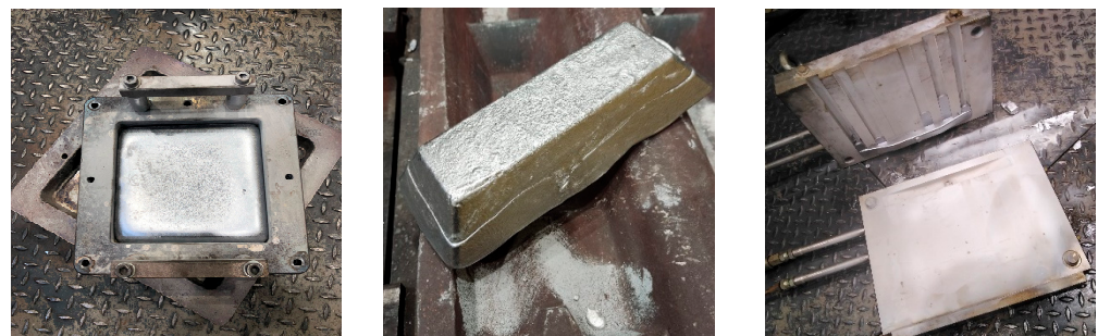
Figure 1. Images of the different samples taken for the tests: square plate (left), small ingot (middle) and flowability test specimen (right).
