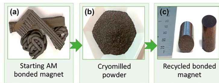
Figure 11. (a) Starting AM bonded magnets (65 vol% NdFeB in nylon), (b) cryomilled powder, and (c) recycled bonded magnets. Reprinted with permission from ref. [127]. 2019, ScienceDirect.
