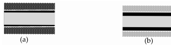
Figure 12. Schematic diagram showing effects of die temperature and plunger speed on solidified layer thickness with 1 mm die gap. (a) Die temperature: 30 °C, plunger speed: 0.2 m/s. (b) Die temperature: 150 °C, plunger speed: 0.8 m/s.
