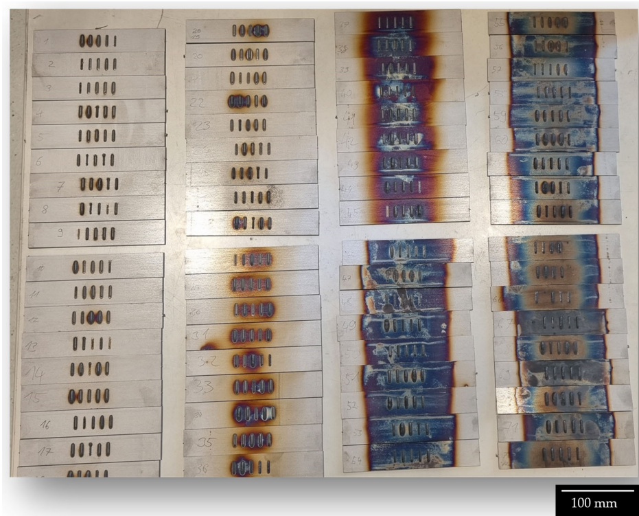
Figure 3. Produced samples sorted in ascending bins by substrate temperature in a zig-zag-fashion (start: upper left corner → down → right and up).
