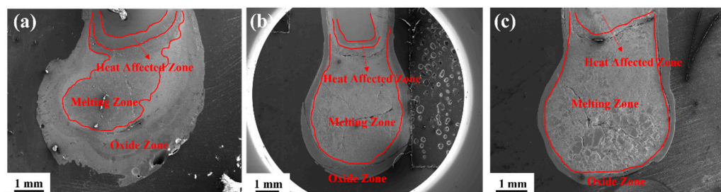
Figure 6. SEM BSE micrograph showing morphology of \text{Ti}_{100-x}\text{Zr}_x alloy post-combustion: (a) \text{Ti}_{70}\text{Zr}_{30} alloy, (b) \text{Ti}_{50}\text{Zr}_{50} alloy, and (c) \text{Ti}_{70}\text{Zr}_{30} alloy.
