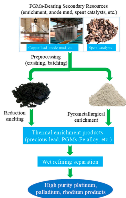
Figure 6. Traditional pyrometallurgical process flow chart.
