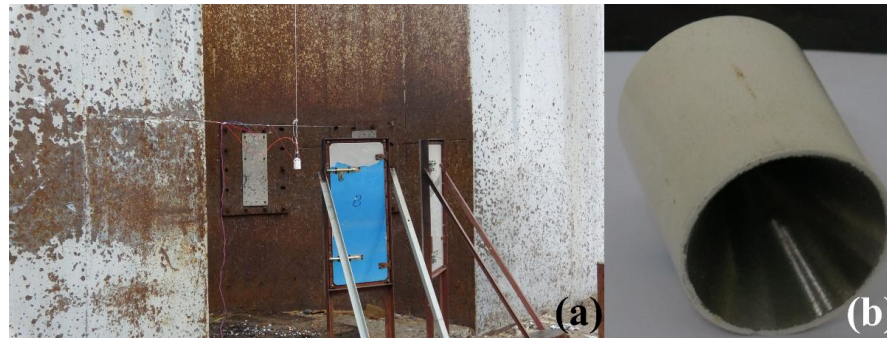
Figure 2. Jet formation X-ray experimental setup. (a) X-ray experimental setup, (b) SC structure.
