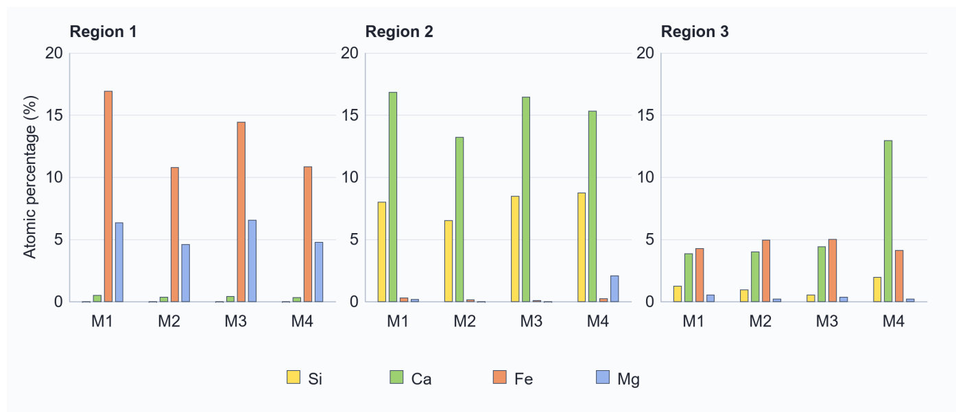
Figure 14. Local EDS comparison for the MgO series; O is omitted to highlight Si, Ca, Fe, and Mg.
