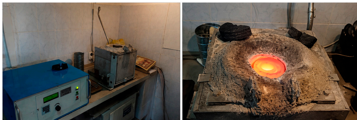
Figure 2. Induction furnace during the smelting of a nickel–chromium-containing ferroalloy.
