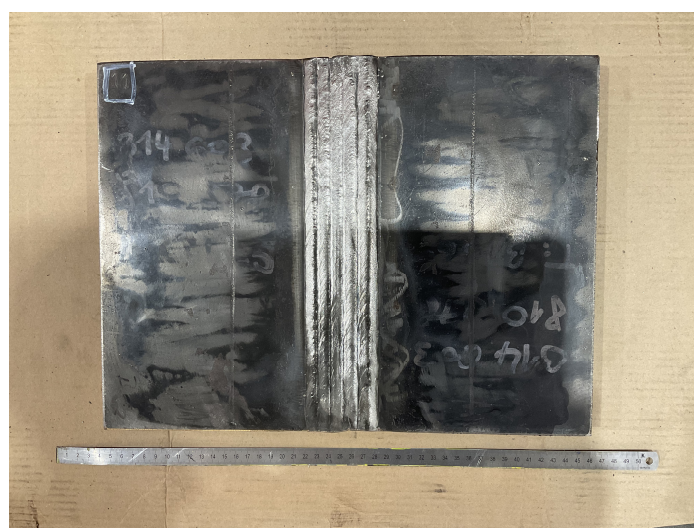
Figure 1. A picture of the welded sheet.
