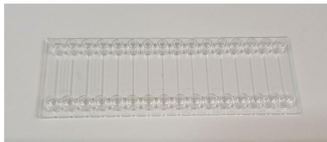
**Figure 4.** Example of a polymer transfer standard chip.
