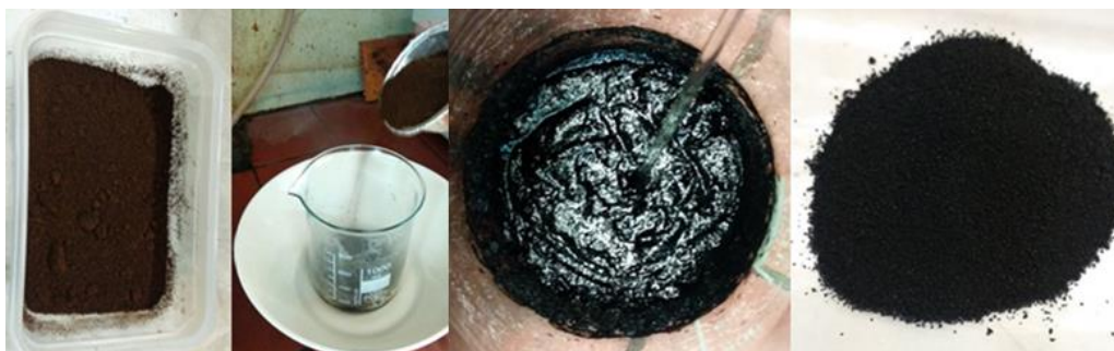
Figure 2. From left to right: spent coffee carbonization in piranha solution, followed by washing and drying, led to a fine carbon powder (codenamed SCPS) with a yield of 35%.
