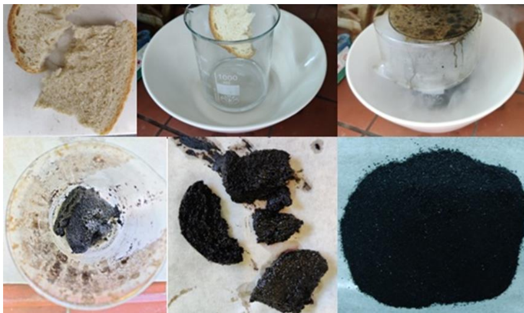
Figure 1. From top-left to bottom-right: stale bread carbonization in piranha solution, followed by washing and drying, led to a fine carbon powder (codenamed BRPS) with a yield of 25%.
