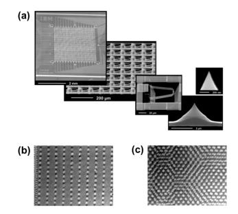
**Figure 14.** (a) SEM images of the IBM Millipede, which contained an array of 1024 cantilever tips, each with an integrated heater-thermometer above the tip [30]. (b,c) Data bits with aerial densities of up to 400 Gbit/in<sup>2</sup> written on polymer thin-films using the Millipede [203].
