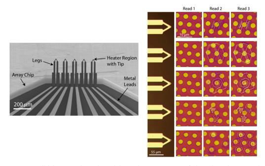
**Figure 15.** Parallel thermomechanical nanolithography using an array of 5 heated cantilevers. Read 1: thermal image of the substrate. Read 2: after first cycle of lithography. Read 3: another lithography cycle at lower writing temperature to pattern lower and narrower features [178].
