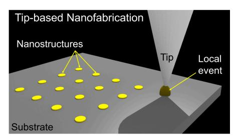
**Figure 1.** A cartoon illustration of tip-based nanofabrication. A tip is brought into close proximity with a substrate. An external stimulus to the tip results in a physical or chemical event localized to the tip-surface junction resulting into the fabrication of a nanostructure. The tip is then moved to the next position to fabricate the next structure.
