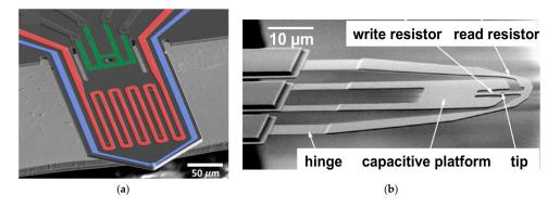
**Figure 13.** (a) SEM image of the cantilever with thermal bimorph actuation (red), piezoresistive sensor (green), and electrode to the conducting tip (blue). A cantilever is used for advanced electric-field scanning probe lithography on molecular resist [183]. (b) Heated cantilever with a capacitive platform for electrostatic actuation, heated tip, and resistive read sensor [155].
