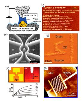
**Figure 5.** (a) Schematics illustrating local oxidation of a metal surface. (b) First paragraph of "Don Quixode" defined by LON. (c) AFM image of a quantum ring fabricated by LON. (d) Quantum dot defined by local oxidation. (e) Silicon nanowire transistor fabricated by LON and the drain current versus drain voltage at different gate voltage setting. (f) Superconducting 4 nm thick niobium nitride (NbN) nanowires defined by local anodization.
