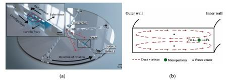
**Figure 4.** (a) 3D representation of the design with an illustration of forces affecting a fluid element passing through the channel. The channel size is exaggerated for demonstration purposes. (b) A cross-section in a rectangular spiral microchannel showing the direction of Dean vortices and the forces affecting microparticles flowing in that channel.
