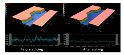
**Figure 2.** A 3D reconstruction of the fabricated channel showing the difference in surface roughness before and after the glass etching process. The arithmetic average values for the roughness profile ( $R_a$ ) are 0.6755  $\mu$ m and 0.4571  $\mu$ m before and after glass etching, respectively.
