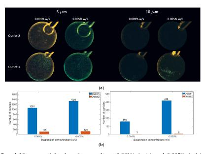
Figure 5. 5 and 10  $\mu$ m particles focusing results at 0.001% (w/v) and 0.005% (w/v) suspension concentrations. (a) Outlet chambers after particle fractionation experiments. (b) The effect of particle suspension concentration on focusing efficiency for 5  $\mu$ m particles (left) and 10  $\mu$ m particles (right). Results show that higher concentrations return higher throughput while approximately maintaining the same focusing efficiency.
