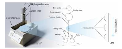
**Figure 1.** Three-dimensional (3D) illustration of the spinning system with all its components, and the microfluidic design of the focusing channel. Microchambers are implemented along one side of the focusing channel to enhance particle focusing.
