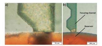
**Figure 3.** Dyed deionized (DI) water flow experiment inside the focusing channel. Picture (a) shows the fluid stopping at the channel inlet due to the pressure barrier caused by the width expansion, while picture (b) is taken after rotating the microfluidic disc at 1500 rpm.
